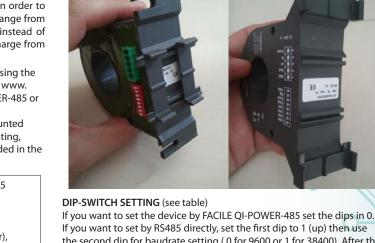
If you want to set the device by RCLL OFFOWLR405 set the dips in 0. If you want to set by RS485 directly, set the first dip to 1 (up) then use the second dip for baudrate setting (0 for 9600 or 1 for 38400). After the settings, please save the configuration by the COMMAND register, then switch off the power supply, before to switch on the power supply set the dips in 0.
