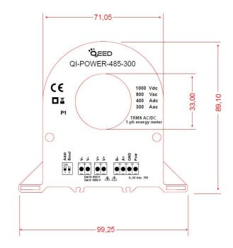
Suitable for measurements with varying frequencies (Wind, Hydro, Shipbuilding Industries, Aviation). Telecom applications, Refrigeration, Motors, OEM's application. Suitable for direct measurements between inverter and motor.
