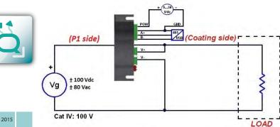
CAUTION: Magnetic fields of high intensity can vary the values measured by the transformer. Avoid installation neal permanent magnets, electromagnets or iron masses that induce strong changes in the magnetic field. If any irregularity recommend reorient or move the transformer in the area most appropriate.
