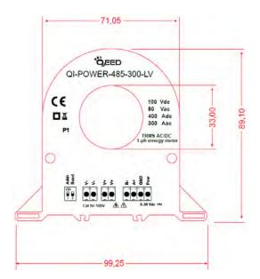
Suitable for measurements with varying frequencies (Wind, Hydro, Shipbuilding Industries, Aviation). DC Motor Control, Telecom applications, Data Centers, UPS, Batteries monitor.
