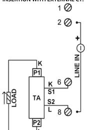
the input Voltage (LINE) has to be connected on terminals 2 (+) and 8 (as for the direct insertion).
