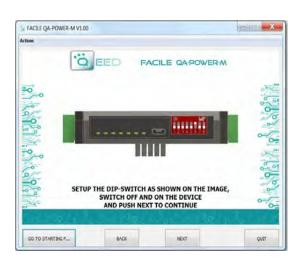
It is possible to use the program without connecting to the module, in this mode you can SAVE the configuration on your PC, which can then be sent to the QA-POWER-M at a later time.
