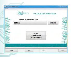
It is possible to use the program without connecting to the module, in this mode you can SAVE the configuration on your PC, which can then be sent to the QA-12DI-4DO at a later time.
